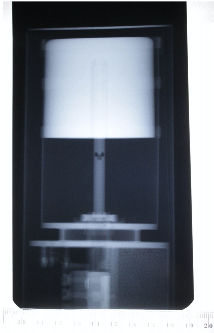
Figure 3.2: Picture of the HPGe detector radiogram (p-type Ortec GEM 35). [1]
