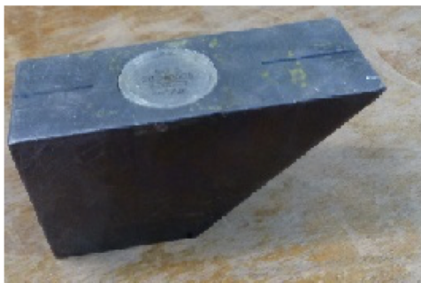
Figure 3.4: The photo (left) and the scheme (right) of the lead collimator for the dead layer thickness measurement. [1]
