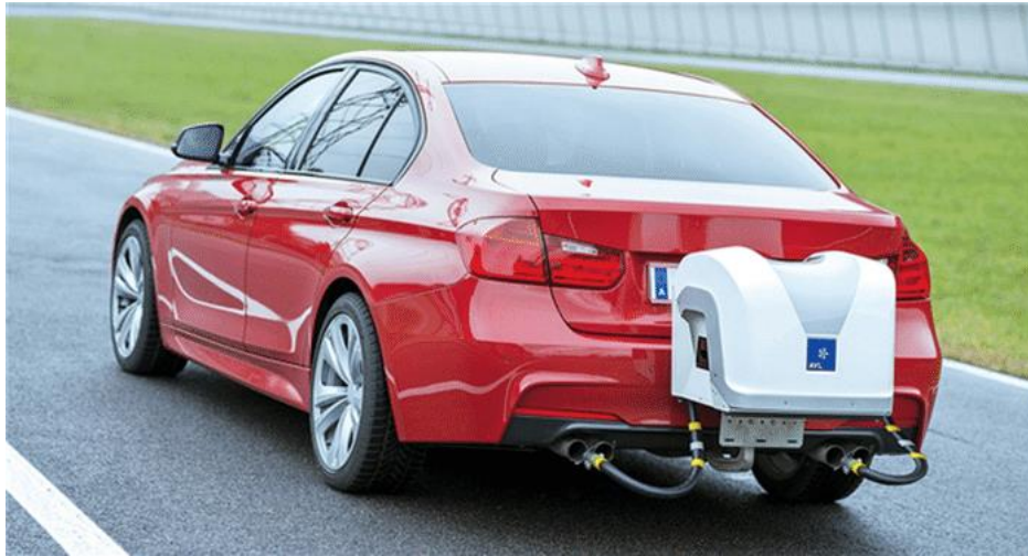
Fig. 13 – PEMS device installed on a test vehicle [21]
