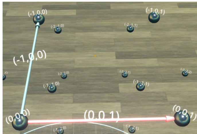
Figure 5.13: Visualization of vector rotation around the y -axis by 90^\circ
