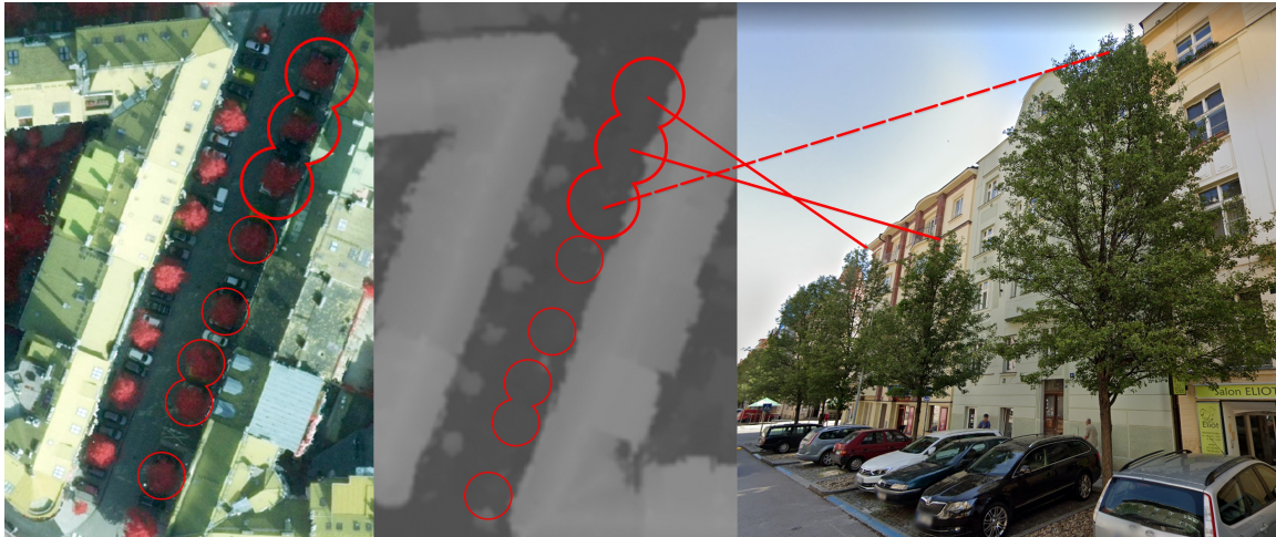
Figure 5.1: Mistakes in the DSM. Clearly visible trees from the CIR imagery (Left), completely filtered out trees from the DSM (Middle), and the image from the street (Right).
