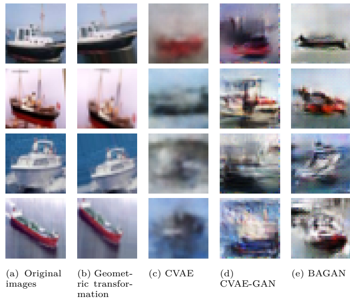
Figure 6.1: Visualisation comparison of original images (a), geometrically transformed images (b) and images generated by CVAE (c), CVAE-GAN (d) and BAGAN (e). The models were trained on data with 50% of the minority-class missing.
