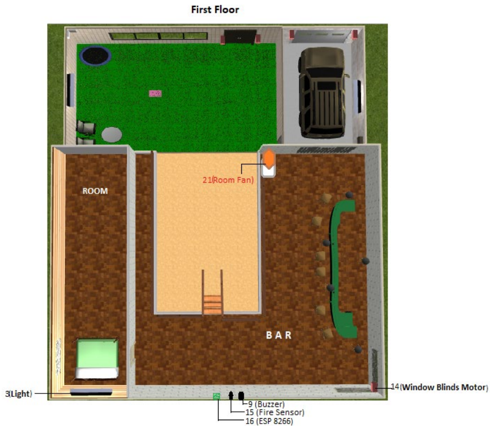
Figure 17: Placement of the electronics devices on First Floor
