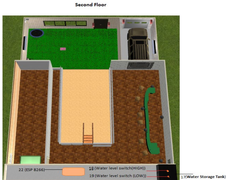
Figure 19: Placement of the electronics devices on Second Floor
