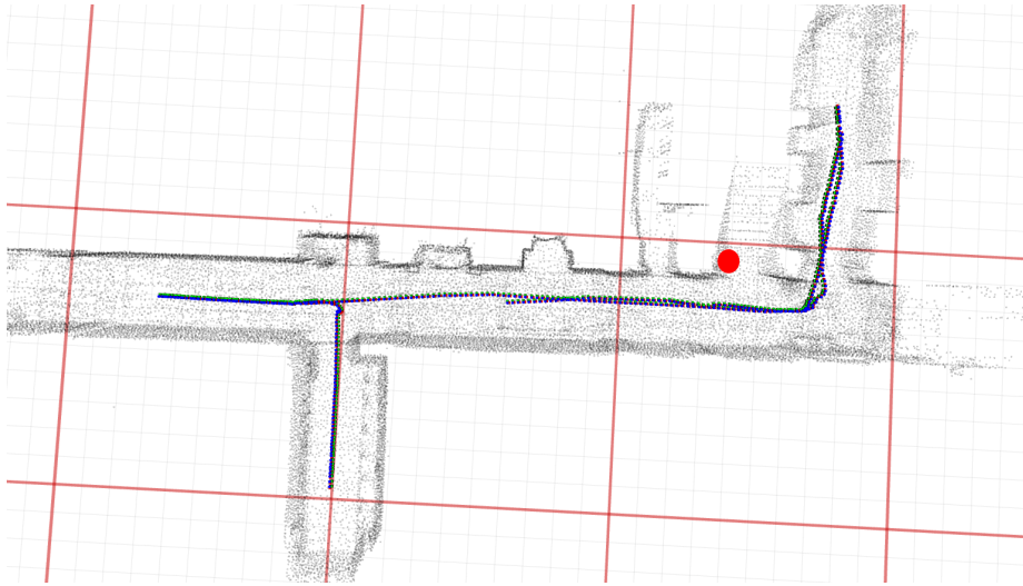
Figure 18: Robot map and path around a corner, with phone on the right corner
