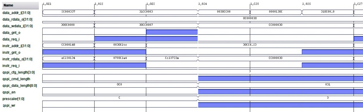
Figure 4.6: RISCv PULP bus transactions measured by internal FPGA Vivado logic analyser.
