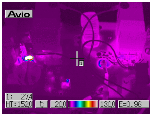
Figure 4.8: Temperature measurement with NTC at 1.5 kW
