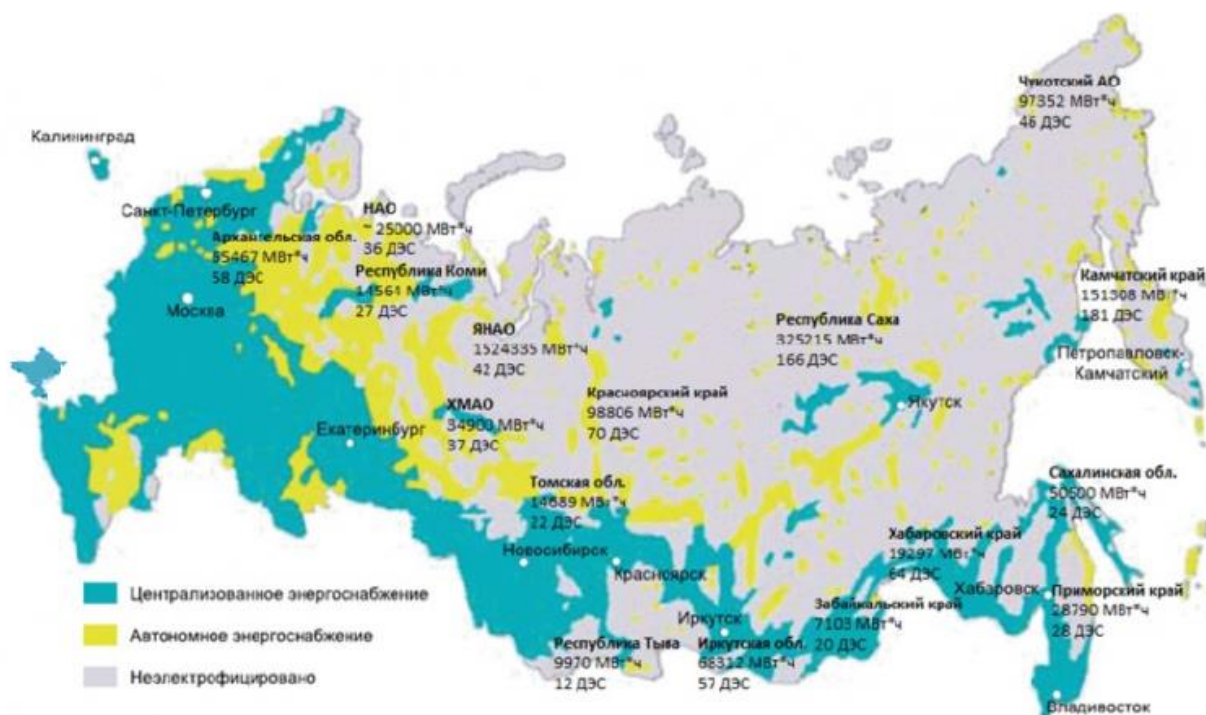
Figure 29 – Map of Russian electricity grid with information on amount and production of local municipal diesel power stations [35]
