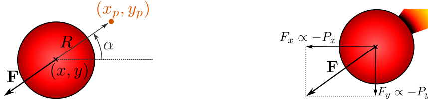
(a) Acoustophoretic force created by a high-pressure point (represented by orange color). (b) Acoustophoretic force created by a gradient of acoustic pressure (represented by color gradient in the upper right corner).
