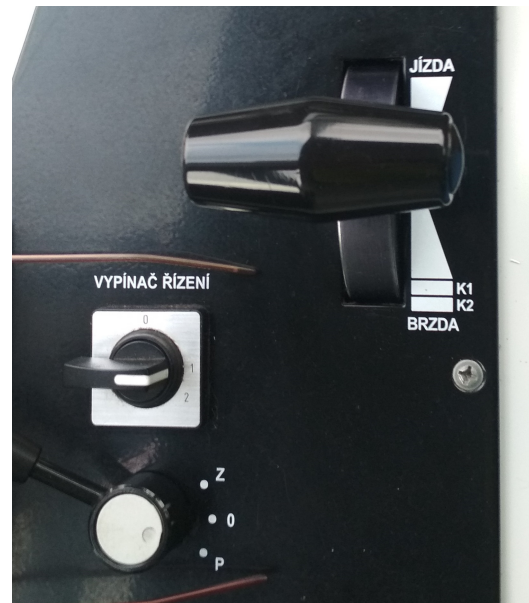
Figure 5.2: The control lever from the VarioLF tram used in Ostrava experiments.
