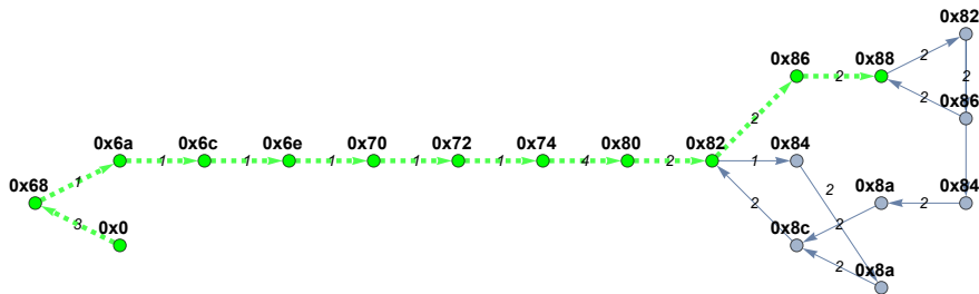
Figure 6.3: Worst case execution path to specification rule 5 visualised using Wolfram Mathematica. The path marked in green with edges dashed shows the worst-case satisfaction path output by the checker.
