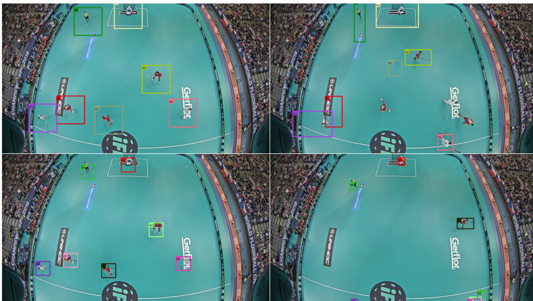
Figure 4.7. Visualization of tracking by the DiMP tracker. The first row shows the initial frame with bounding boxes of size 200. The second image is tracking after 39 frames. The second row shows the same situation with bounding boxes of size 150.
