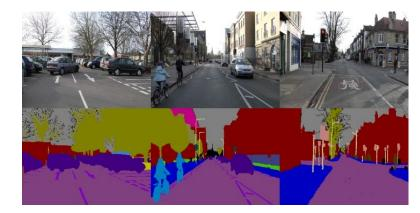
Figure 1.1: Example of car-mounted camera image semantic segmentation reproduced from [BFC09]
