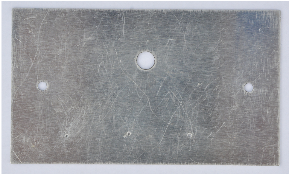
Figure 6.5: Testing sheet of metal with artificial flaws
