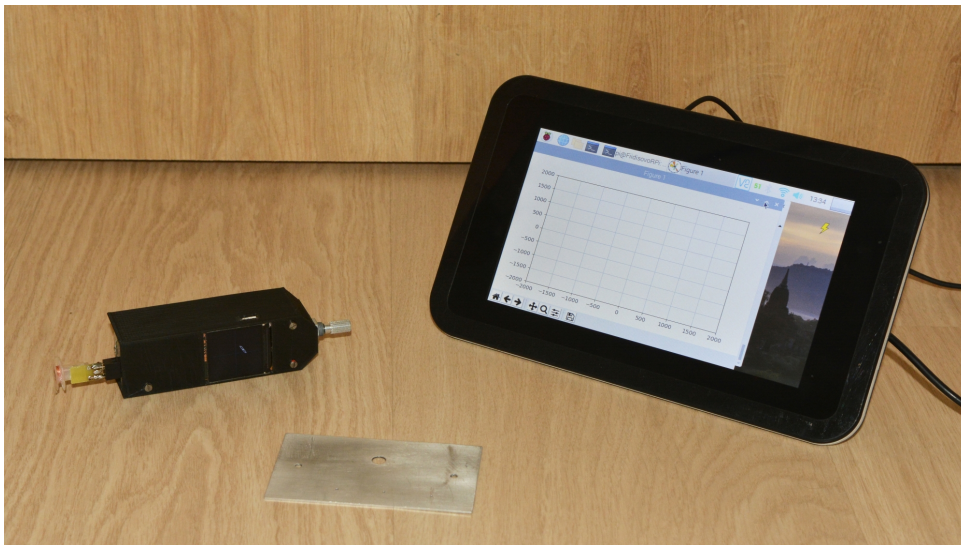
Figure 6.4: The ECT measurement system
