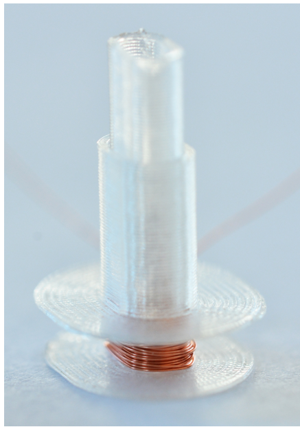
(a) : Wounded TX coil on a 3D printed frame
