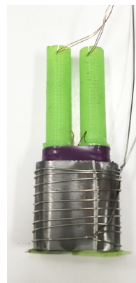
(b) : RX coils with shielding
