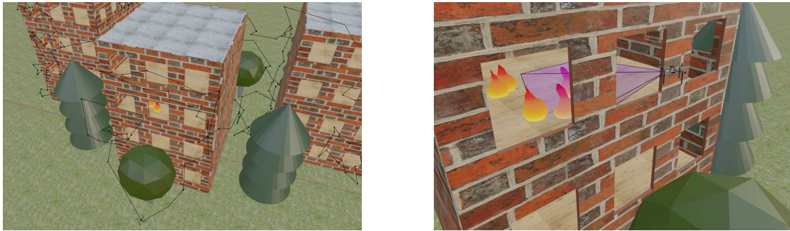
Figure 1.1: Illustration of the method’s function in a housing estate – the left figure depicts an example of a final inspection path, the right figure illustrates the sensor’s field of view during the fire detection
