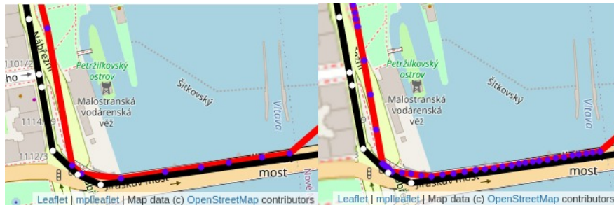
Figure 4.1: Difference between unprocessed GPX (left) and GPX with evenly spaced points added between each two succeeding GPX points (right).
