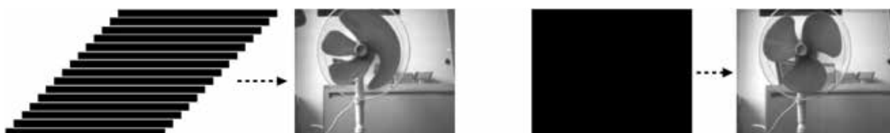
Fig. 10. The moving fan blade continues to turn as lines are read out sequentially resulting in characteristic rolling shutter distortion. By reading out all pixels simultaneously, a global shutter sensor captures the fan without any distortion.
