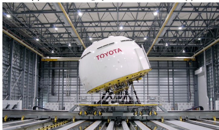
(b) : Toyota hexapod architecture 6 DoF simulator with moving base for motion envelope extension [9]
