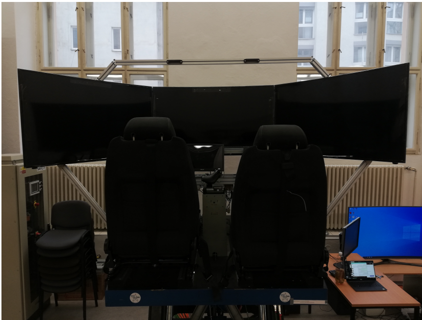
Figure 3.5: 3 TV visualisation setup
