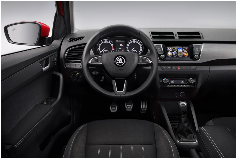
Figure 2.2: Skoda Fabia interior with all driver input devices: steering wheel, pedals, handbrake, gear shift [2]
