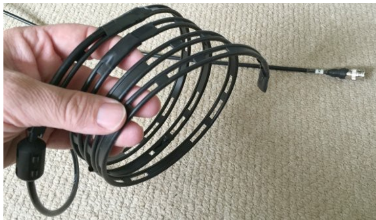
Figure 4.9: A roll-up slim jim antenna. Source: [L20]
