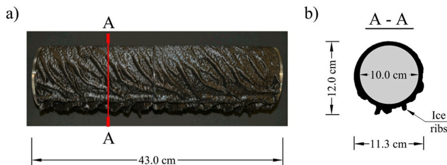
Fig. 7. (a) The simulated-ice-accreted cable model reproduced for aerodynamic investigations on a scale of 1:1.6 using the 3D Fused Deposition Modeling method and (b) a selected cross-section with the main dimensions.
