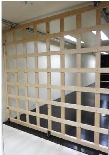
Fig. 11. View of the wooden turbulence grid in the aerodynamic chamber of the wind tunnel.
