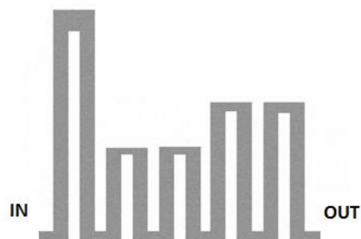
Fig. 1.3: Connected C-sections with different lengths [18].
