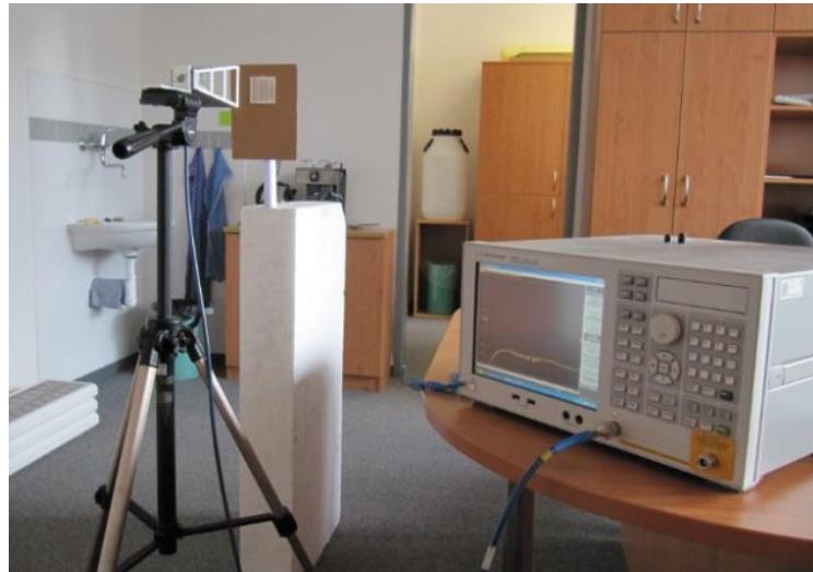
Fig. 6.26: Setup using monostatic configuration for indoor measurement with detail of 20-bit tag constituted by dipoles closely coupled to a rectangular metallic plate attached to a wooden plate.
