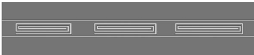
Fig. 1.12: Spiral resonators coupled to coplanar waveguide [72].
