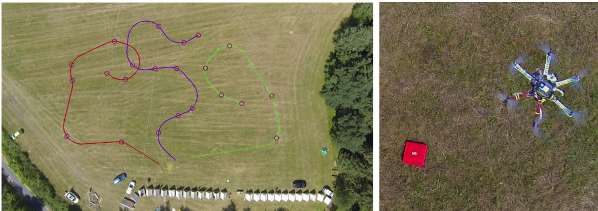
Figure 2.4: Solution of the Multiple Dubins Traveling Salesman Problem obtained by the VNS-based method [4c].
