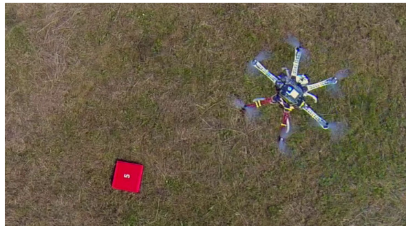
Fig. 7. Hexarotor UAV during the visual data collection of the colored target object with displayed reward.
