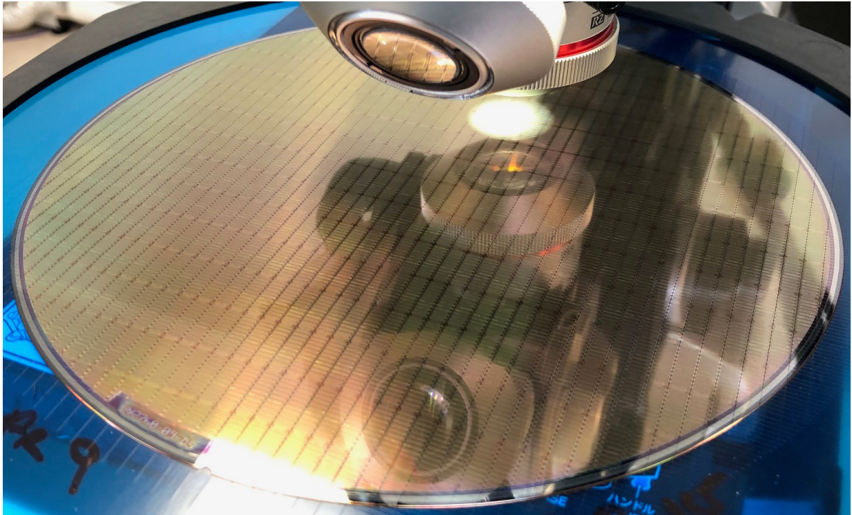
Figure 11.2: A dozen wafers contain approximately 70 000 chips of the PH series.
