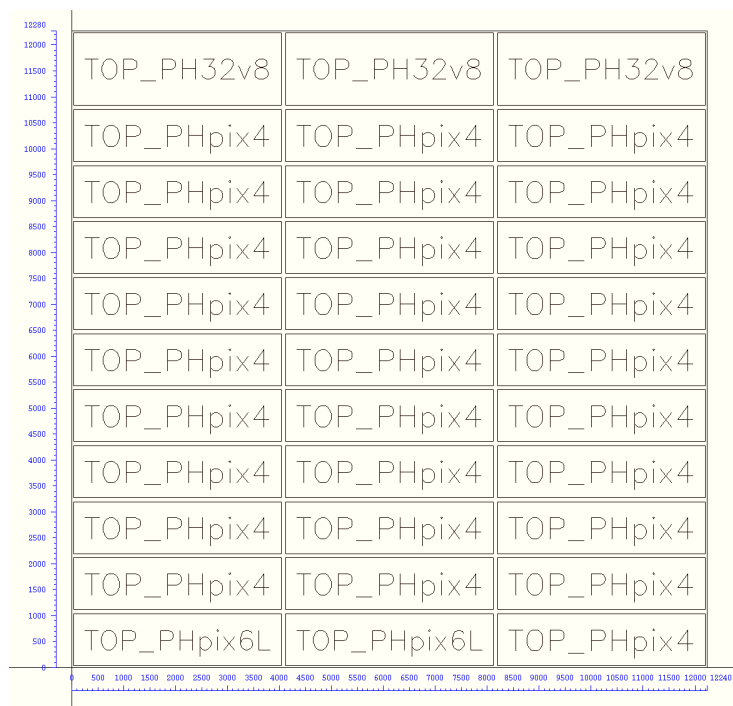
Figure 10.2: One reticle for engineering run with appropriate layout. Reticle dimensions: 12.28 \times 12.24 \text{ mm}^2 .
