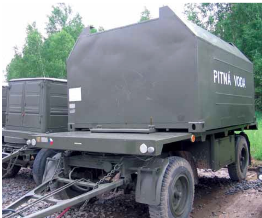
Obr. 8.1.4.1 Cisterna na pitnou vodu CPV-3 [16]
