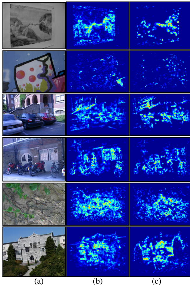
Figure 3.10: Heatmaps for Saddle and ORB detections. Column (a) shows the original images, columns (b) and (c) show heatmaps for Saddle and ORB, respectively. Heatmap represents the number of interest regions current pixel belongs to. The heat pseudo-color indicates the final countings along the feature sets.
