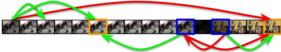
Figure 4.9: Linear and binary search of the SSD algorithm. Arrows on top indicate the forward step for finding the widest frame interval (orange squares) where the potential transition is located. Arrows below indicate the binary search to find tighter transition boundaries (blue squares). The correctly matched images are indicated with green arrows, otherwise in red.
