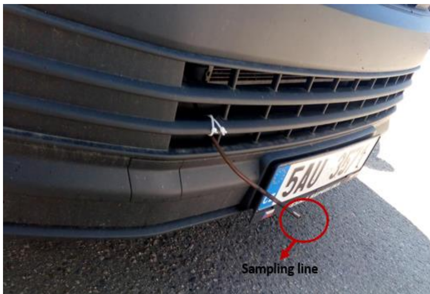
Fig 3.2 Sampling line installed to collect exhaust Plumes from the vehicles
