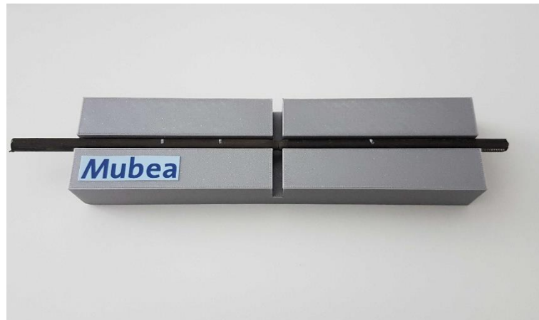
Figure 20: Mubea simple fixture (made using 3D printing)
