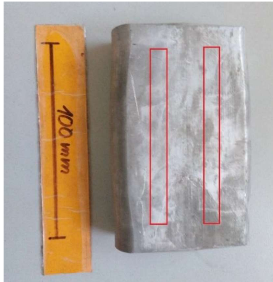
Figure 20 - Place of sampling for the tensile test
