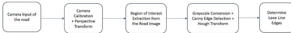
Figure 6: The lane detection system uses the principle of Hough transform and Canny edge detector to detect lane line form real-time camera images(Image is taken from Wikipedia)
