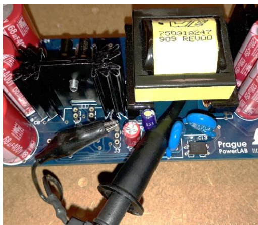
Figure 36 Indirect transformer voltage measurement
