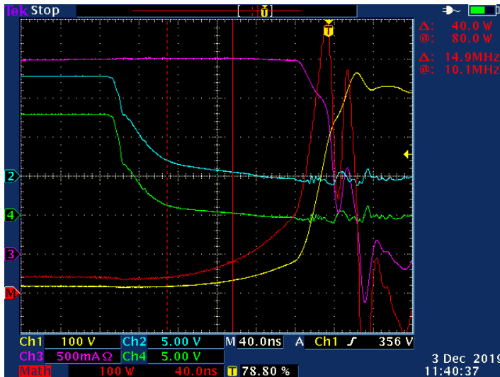
Figure 44 Mos4 switch-off with 1\Omega gate resistor; Ch1 – Drain, Ch2 – Gate, Ch3 – Drain current, Ch4 – Gate Drive, Math – Ch1-Ch3
