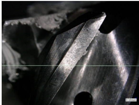
Figure 56: Workpiece Material Clung on the Cutting Tool due to Heat Accumulated on the Cutting Edge.
