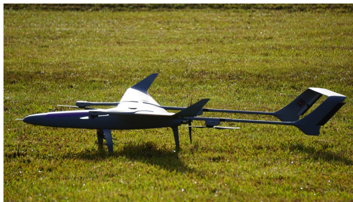
Figure 1.1: [1]: Carbonix Volanti: fixed wing carbon composite industrial drone
