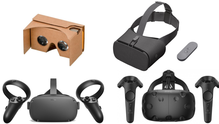
Figure 2.1: Examples of various contemporary virtual reality systems. Clockwise from top: Google Daydream View (mobile), HTC Vive (PC), Oculus Quest (standalone), Google Cardboard (mobile).
