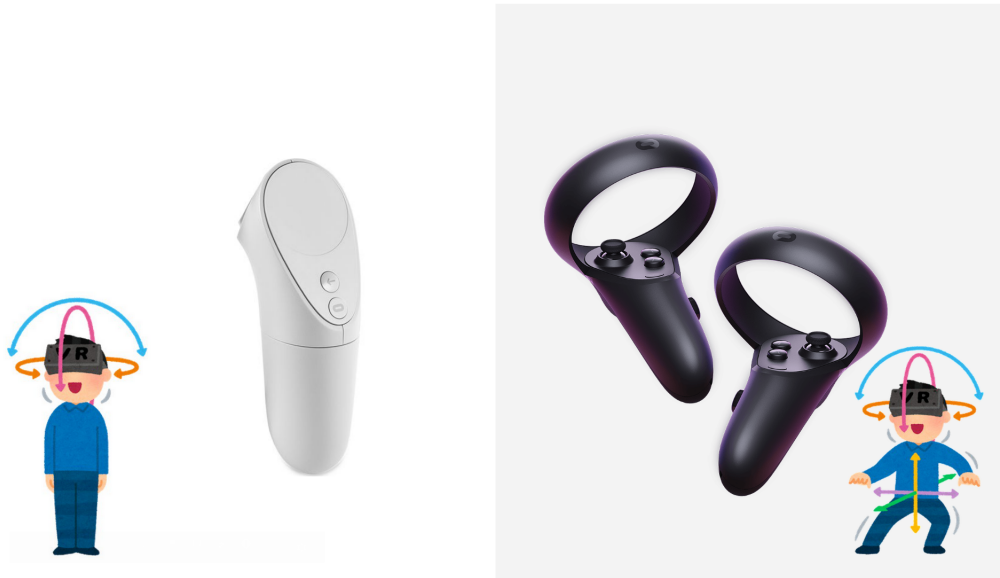
Figure 2.2: Left: Oculus Go controller offering 3 degrees of freedom. Right: Oculus Touch 6DOF controller.[72]
