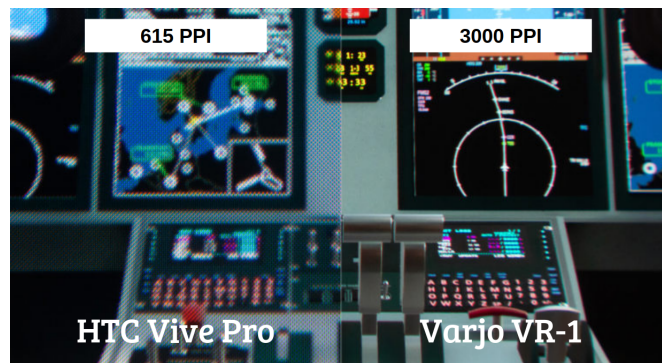
Figure 3.8: Comparison of pixel density between a high-end consumer headset and a business-oriented HMD.[66]
