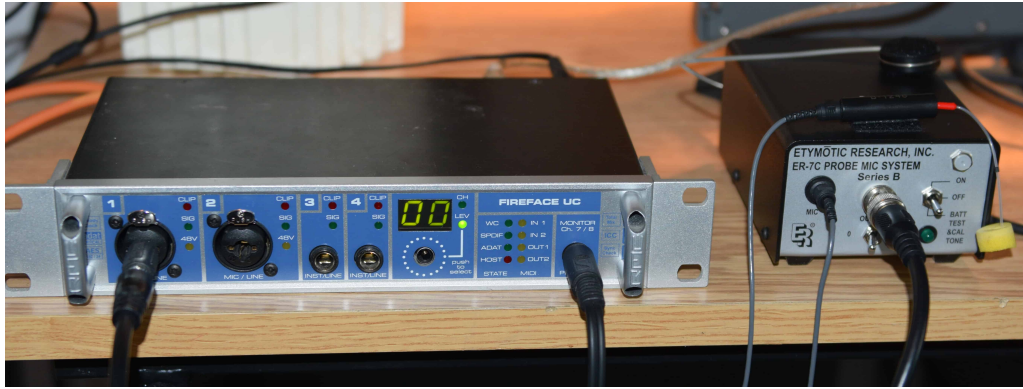
Obr. 3.2: Vlevo zvuková karta RME Fireface UC, vpravo Microphone Probe ER-7C Series B.
