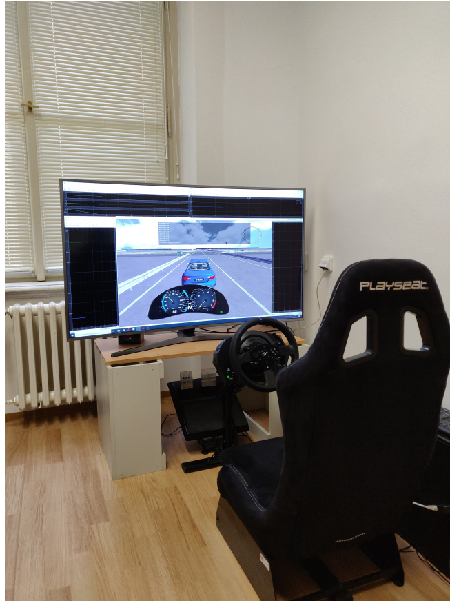
Figure 6.8: Platform used for virtual riding tests.
