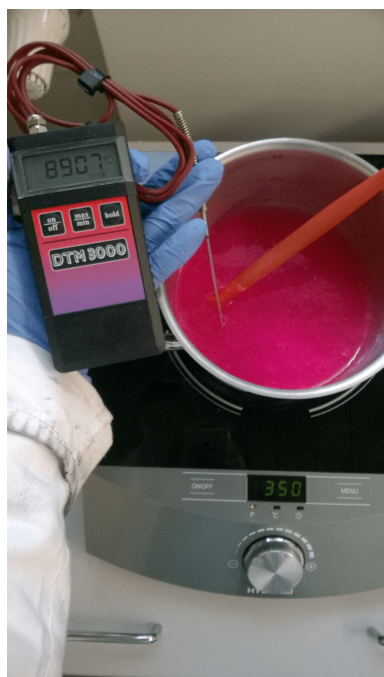
Figure B.9. At temperature above 85 °C, agar solidify and PE powder can be mixed in.
