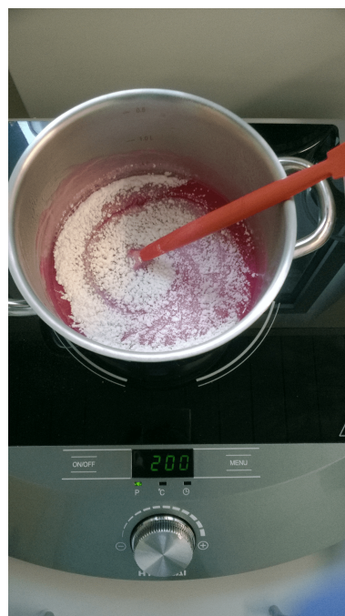
Figure B.10. Sprinkling and mixing polyethylene powder.
