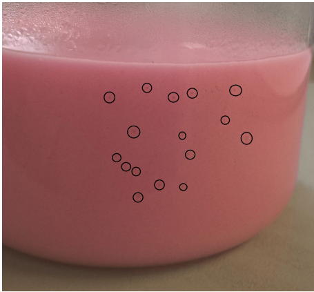
Figure 8.3. Detail of the mixture with marked out air bubbles right after preparation.
