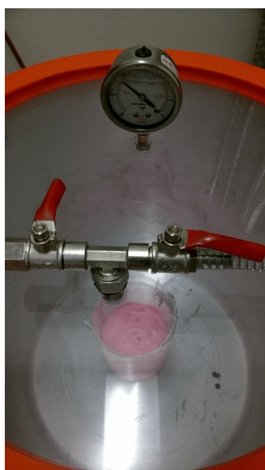
Figure B.11. Use of vacuum system to remove air bubbles from the mixture.
