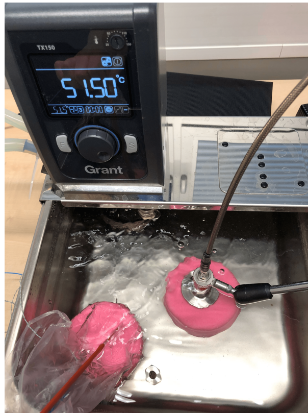
Figure 6.4. Actual measurement setup of temperature dependence of dielectric properties.
