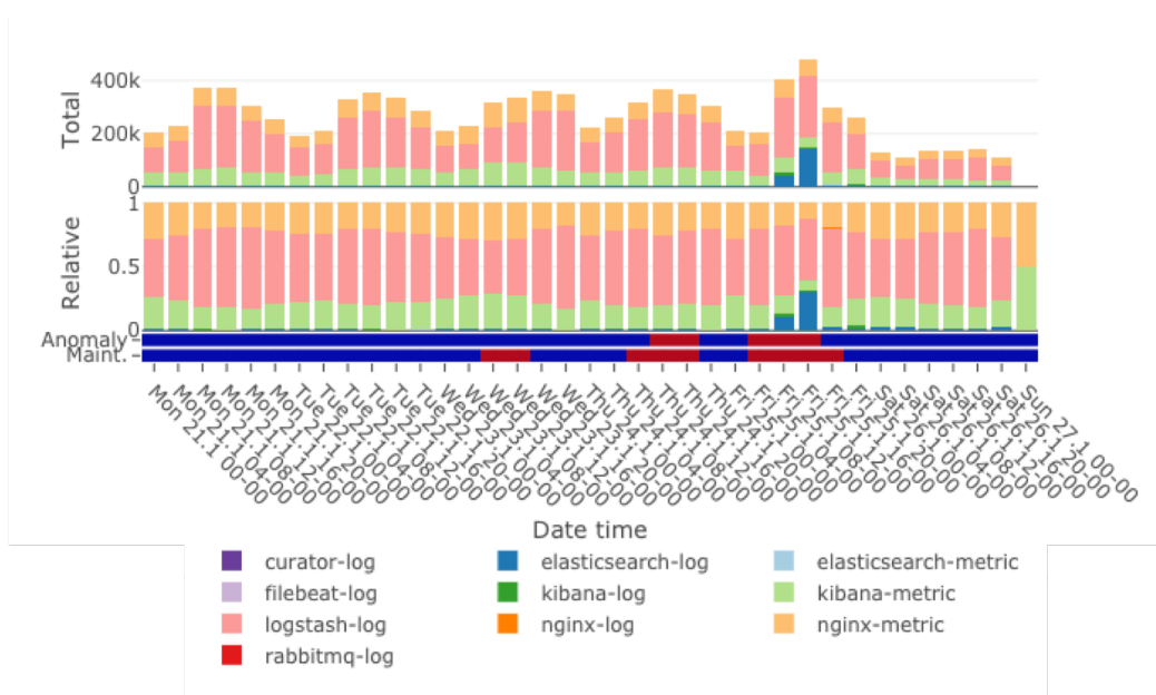
Figure 4.4: Visualization of dataset 2 - a chart of total counts of log and metric records per application per 4 hours in the first part, the second part expresses the same relatively. Under both subplot, there is a visualization of anomaly behaviour and maintenance job labels (red labels an anomaly/maintenance label within the 4 hour range).
