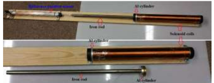
Fig. 12. Measurement set-up for a pneumatic position sensor
