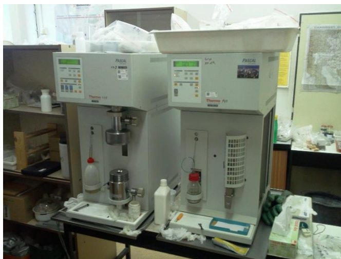
Obr. 41: Rtuťové porozimetry Pascal 140 a Pascal 440 (Thermo Scientific)
