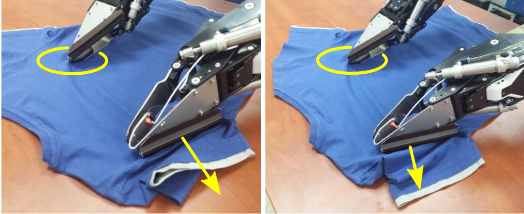
Figure 4.9. The brush tool attached to the gripper is moved in the direction shown by the arrow. The other arm is holding the T-shirt to prevent it from sliding.
