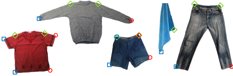
Figure 4.5. Blue squares denote the possible lowest hanging points for randomly grasped garment of a particular category. Red circles denote the symmetric lowest points. Green diamonds denote the desired points to be held after unfolding.
