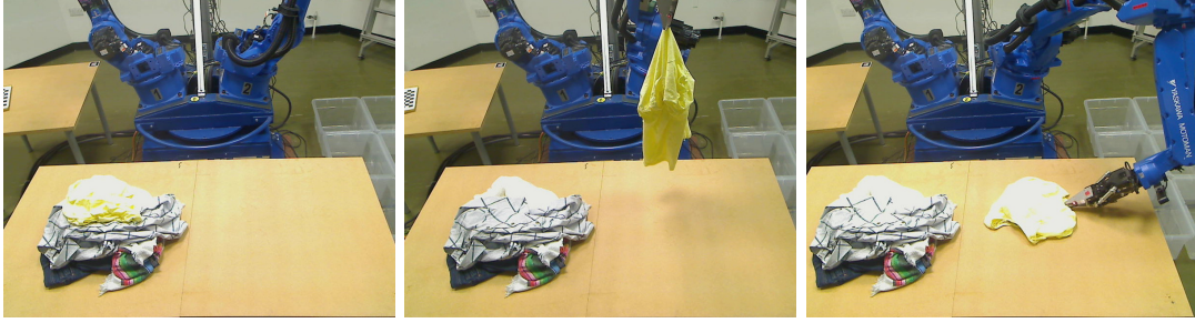
Figure 2.4. [Sun et al., 2016] manipulate the garment actively in order to classify its category from multiple configurations. © 2016 IEEE
