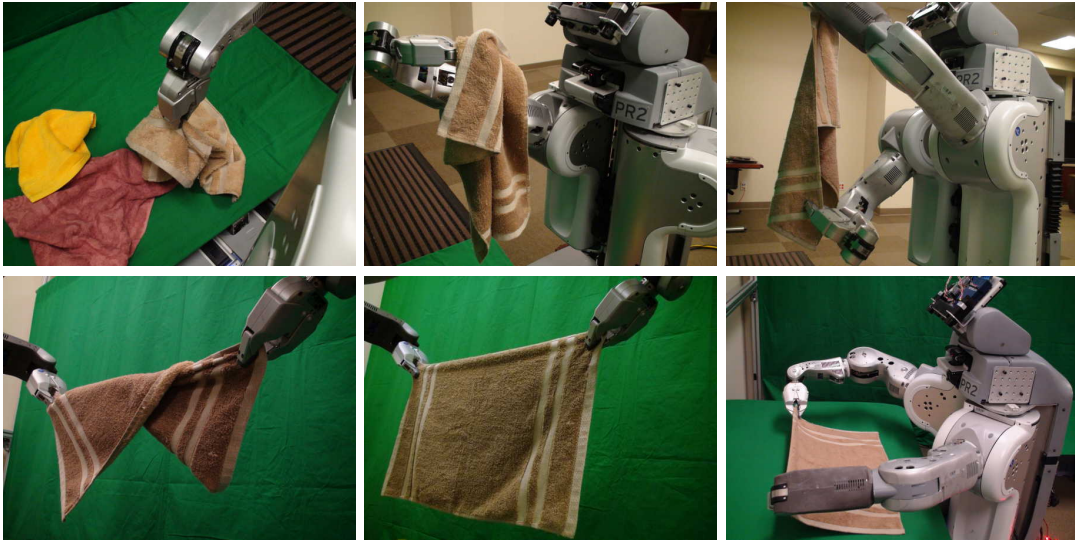
Figure 2.6. [Maitin-Shepard et al., 2010] unfold a towel in a series of manipulations, including untwisting, utilizing information about the detected hemlines and corners. © 2010 IEEE
