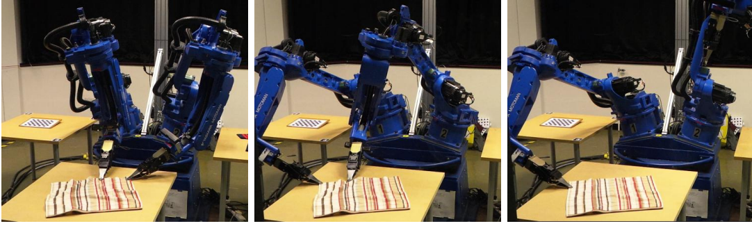
Figure 2.8. [Sun et al., 2015] detect position and orientation of wrinkles on the garment surface. The wrinkles are removed by pulling the garment in the horizontal direction. © 2015 IEEE
