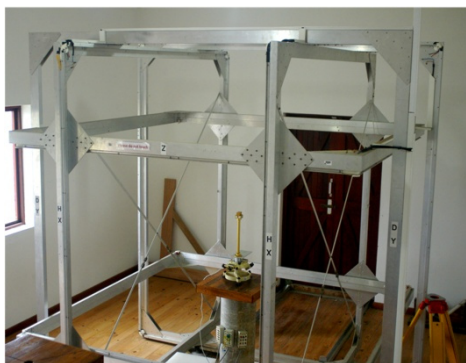
Fig. 1. The square triaxial coil system at SANSa.
