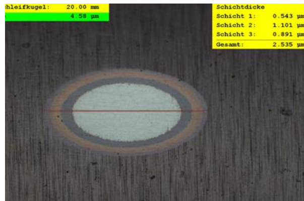
Figure 5-92 Calotest of the best performing AlTiSiN coating
