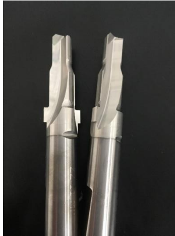
Figure 4-23 TiB 2 coated multipurpose machining tools for aluminum cutting
