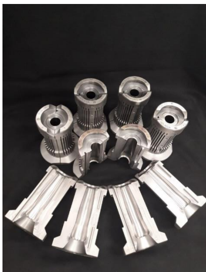
Figure 5-94 Molds after coating
