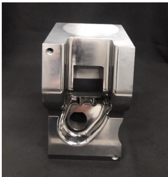
Figure 1-7 Metal forming mold with TiAlCrN coating
