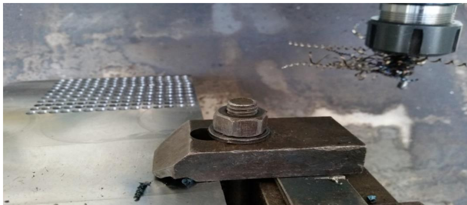
Figure 5-54 Setup of drilling tests with chip
