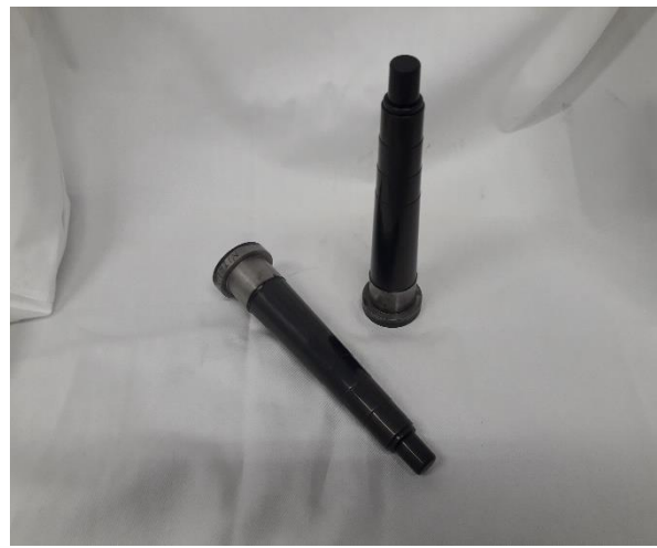
Figure 1-2 Steel mold for HPDC coated with AlTiN
