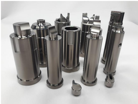
Figure 1-5 Plastic forming pins with CrN coating
