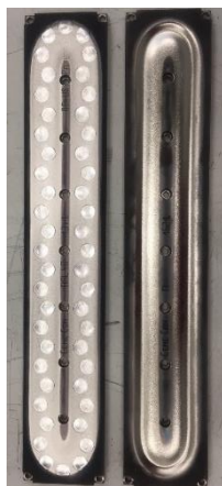
Figure 5-21 Titanium target with aluminum plugs (left) and aluminum target (right) with visible racetracks
