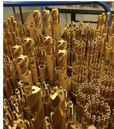
Figure 4-1 Taps coated with TiN coating
