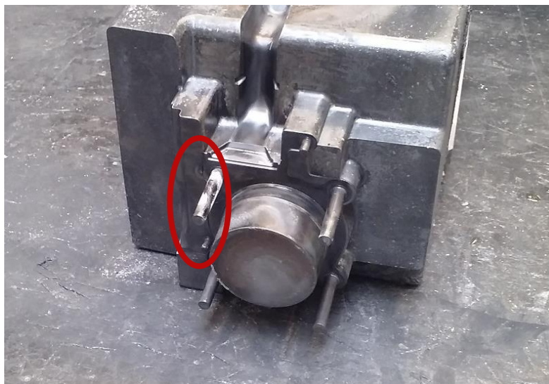
Figure 5-90 Mold core with four coated pins. There is aluminum sticking visible on the stressed pin marked with red color.
