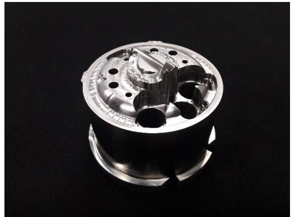
Figure 1-6 Steel molds with TiAlCrN coating
