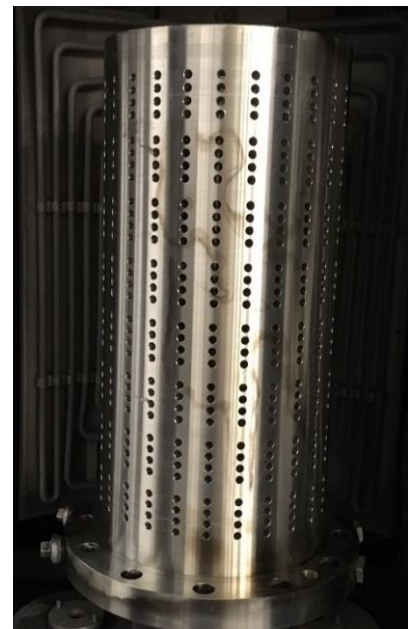
Figure 4-4 Aluminum extrusion cylinder coated with CrN
