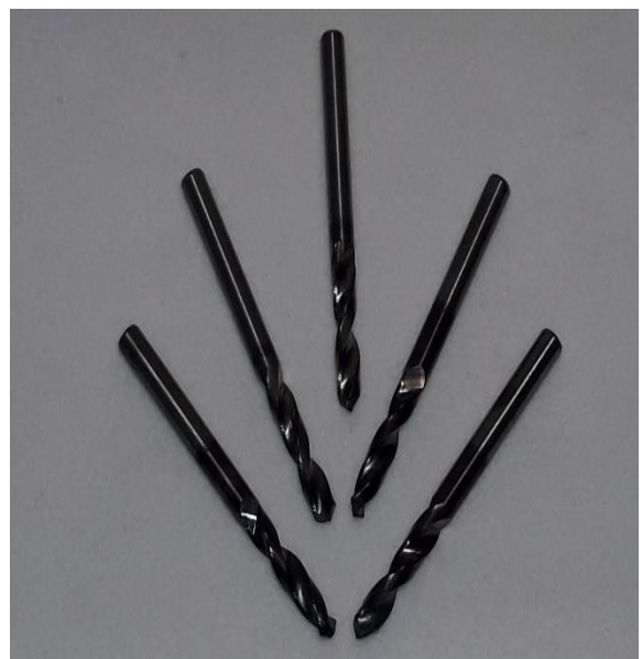
Figure 1-8 Drills with (\text{CrAl})_2\text{O}_3 coating
