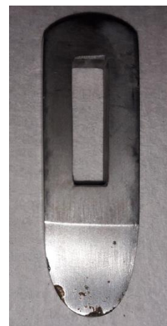
Figure 2-36 Arcing defects on tool steel
