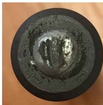
Figure 5-69 Damaged aluminum ball after test
