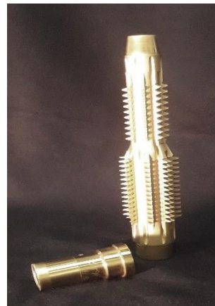
Figure 4-21 TiN coated hob used to produce gears
