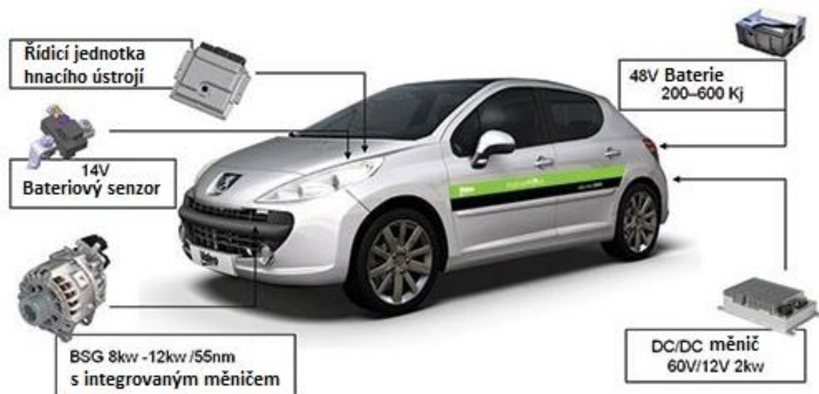
Obr. 4: Valeo 48 V Mild hybrid systém [60]
