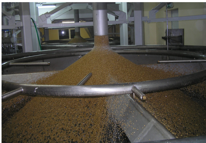
Figure 2.3: Steeping vessel - loading (MOPOS) [3]
