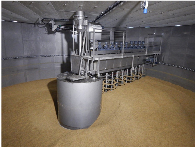
Figure 2.5: Germination circular box with un-/loader and screw turners (MO-POS) [5]
