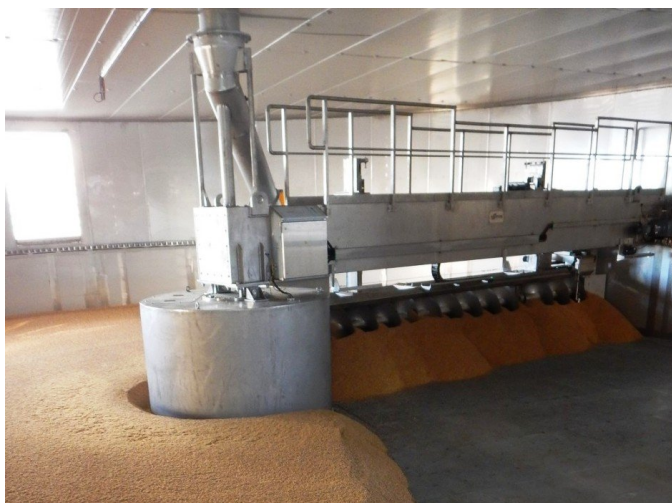
Figure 3.9: Single-deck circular kiln (MOPOS) [10]
