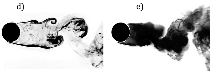
Obr. 9 Vizualizace úplavu za samostatnými válci, a) D = 10 mm, Re = 500, b) D = 10 mm, Re = 1200, c) D = 10 mm, Re = 2500, d) D = 20 mm, Re = 1200, e) D = 20 mm, Re = 2500
