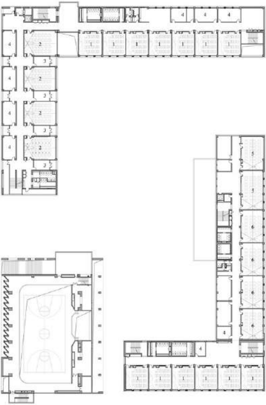
THIRD FLOOR PLAN 1 CLASSROOM 2 LABORATORY 3 PREPARATION ROOM 4 TEACHERS' ROOM 5 HISTORY CLASSROOM 6 COMPUTER CLASSROOM
