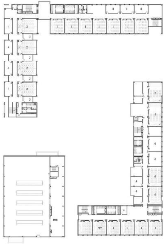
FOURTH FLOOR PLAN 1 CLASSROOM 2 LABORATORY 3 PREPARATION ROOM 4 TEACHERS' ROOM 5 MUSIC CLASSROOM 6 MUSIC CENTER
