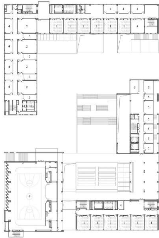
SECOND FLOOR PLAN 1 CLASSROOM 2 LABORATORY 3 PREPARATION ROOM 4 TEACHERS' ROOM 5 ADMIN OFFICE 6 GYM
