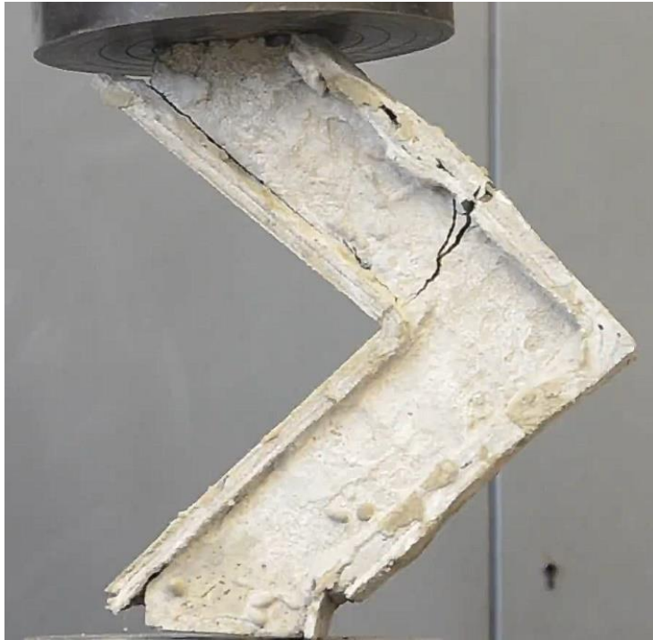
(Fig. 40: Poor bond between TRC and concrete sample. Source: Author)
