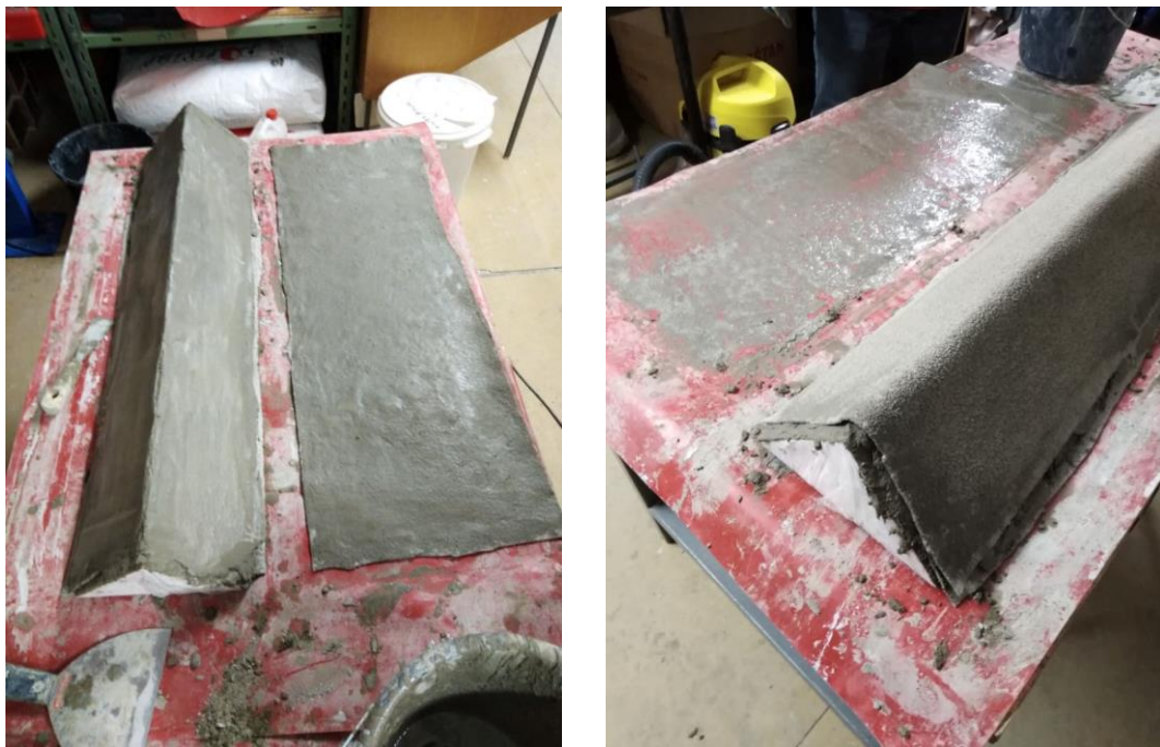
(Fig. 26: Layering of PP textile. Source: Author)
