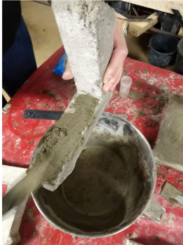
(Fig. 27: Placing extra concrete on RC samples. Source: Author)
