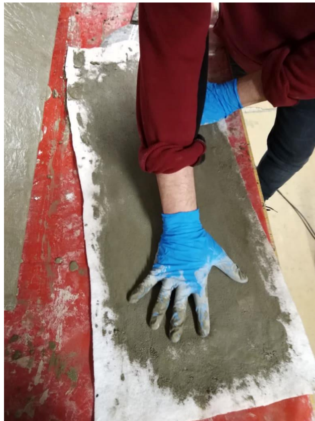
(Fig. 24: Manual rubbing of cement paste to PP Textile. Source: Author)
