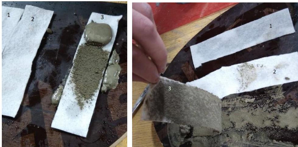
(Fig. 16: PP textile penetration. Source: Author)
