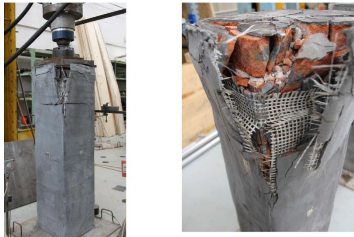
(Fig. 8: Collapsed pillar with TRC protective layer after testing. Source: Holčapek, Vogel and Reiterman, 2019).
