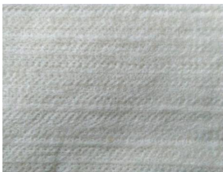
(Fig. 9: Non-woven polypropylene textile. Source: Author)
