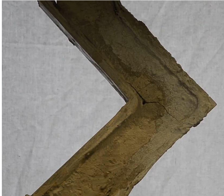
(Fig. 42: First crack during tension. Source: Author)
