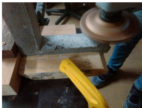
(Fig. 19: Rubbing of samples. Source: Author)
