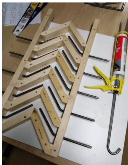
(Fig. 14: Wooden form-work for tension test. Source: Author)
