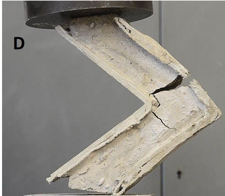
(Fig. 38: Failure of concrete specimen. Source: Author)
