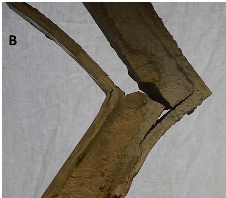
(Fig. 44: Failure of TRC specimen under tension. Source: Author)
