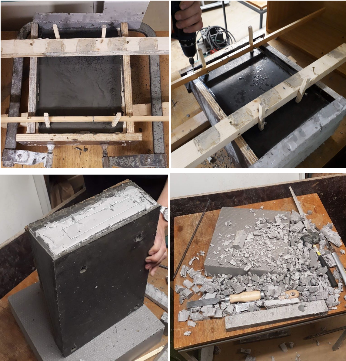
Fig. 24. Concreting and removing of Planter tile form
