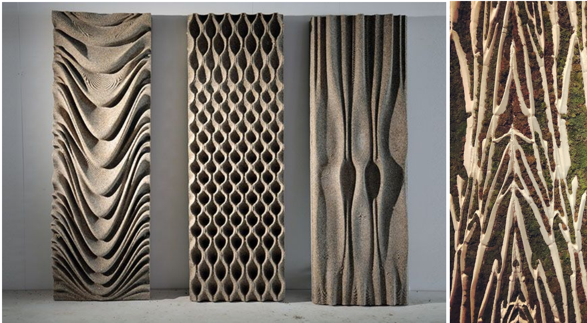
Fig. 4. Bioreceptive concrete panels-BiotA Lab
