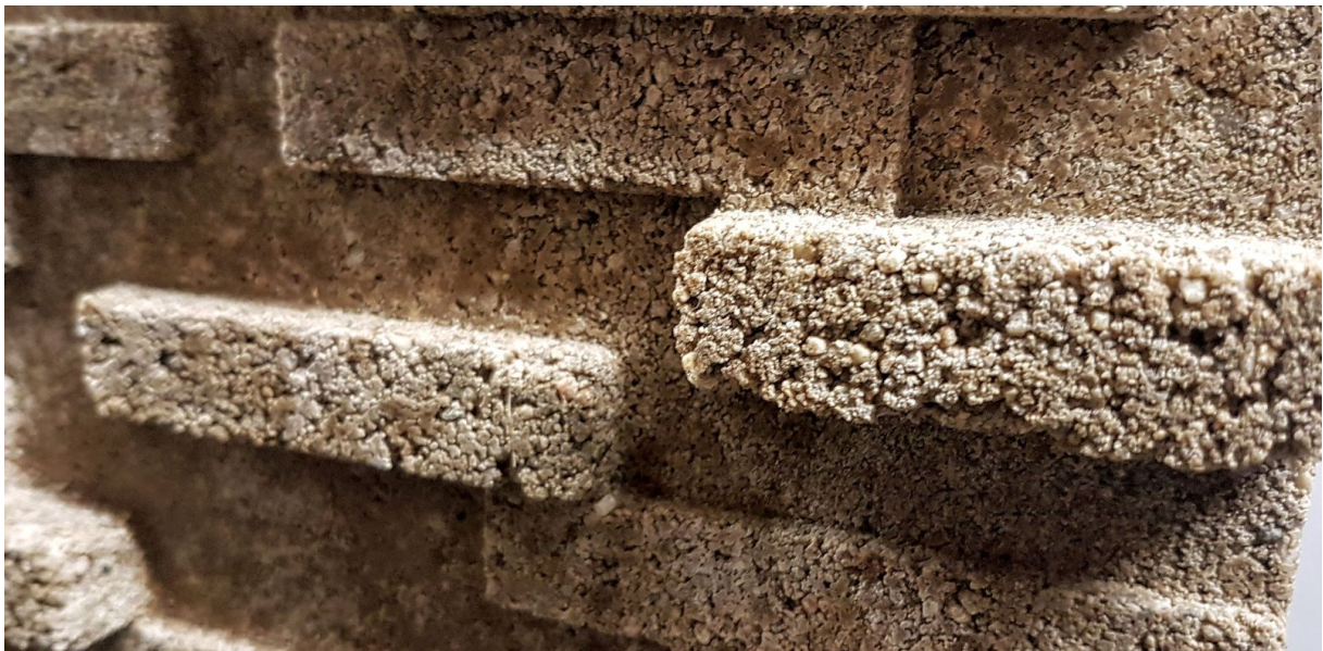
Fig. 26. Rough and porous surface of tile.
